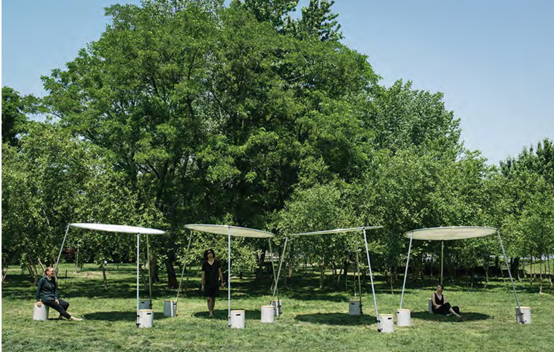
The counterweight offers a seat, back rest, table top, display surface and step stool during set up. The user is invited to feel part of anchoring the unit
