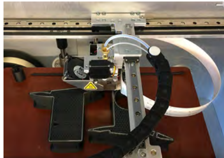
A bracket is born: 3D-printing the joint nodes and brackets at Laufs Engineering | Credit: Eva Jensen Design
